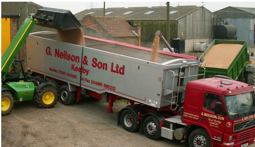
Figure 4. Lorry loaded by auger and front loader
